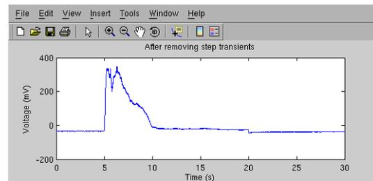
Note for the curious: we measured the recorded voltage  $DI = 4$  samples before and after the step, and subtracted the difference.
