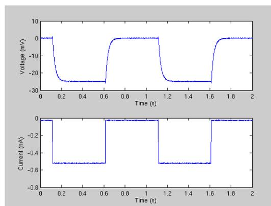
The bottom trace shows the current applied to an RC circuit; the top trace shows the resulting voltage. We are going to determine the time constant of each of the transitions. By zooming into the graphs, it is easy to determine that the transitions occur at 0.12 s, 0.62 s, 1.12 s and 1.62 s. Alternatively, you can use Matlab to find the transitions:
