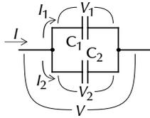
Just as for the parallel combination of two resistors, we have  $I = I_1 + I_2$  while  $V_1 = V_2 = V$ . In this case, that means  $I = C_1 \frac{dV}{dt} + C_2 \frac{dV}{dt} = (C_1 + C_2) \frac{dV}{dt}$ . Thus we can usefully write:
